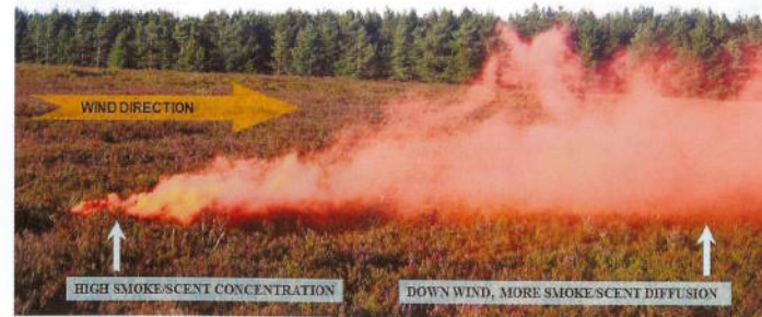
Figure 8 - A scent cone in open air, velocity of the air currents determines the shape and length of the scent cone. (Demonstrated with the assistance of Dave Coss, Ian Bunting and Tyke - Mountain Rescue Team Search and Rescue Dog - of Edale MRT. Image taken by author, 2007)
